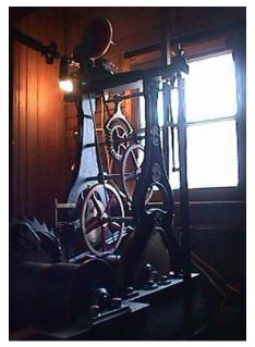
The strike section is unique. Stevens used the count wheel Crane striker system. This is a walking escapement which depends on striking hammer recoil for its control and function.
